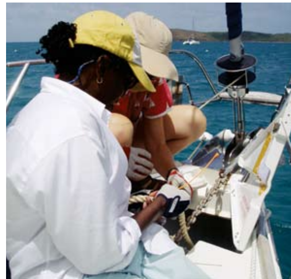
Brightly colored cable ties, readily available at most hardware stores, make great markers for measuring rode length. Adam Colson photo
